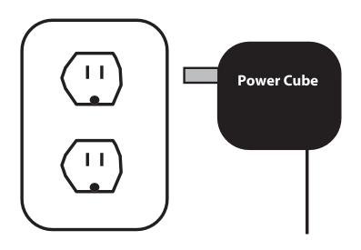
2. Find the power switch on the back of the unit and place it in the "I" position. The status light will begin to flash orange.
