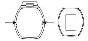
2. To remove the PHB from a bezel place one hand one on each side of the PHB/bezel with the front of the PHB/bezel facing toward you then flex inward.
